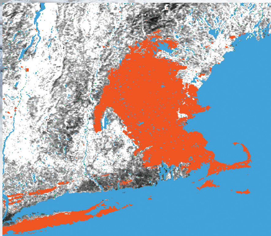
Figure 7: Examples of very dense forests in Canada creating problems with retrieval of the snow cover on the ground. The snow map is from 30 January 2003. The whole area is likely fully snow covered. Blue is open water, red is clouds.
