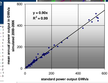
The mean annual power output of 100 hydropower plants was accurately calculated with the model over the years 2000 to 2006.
